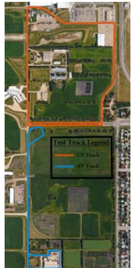
The South Campus CAV test track facility includes one connected vehicle (CV) and one automated vehicle (AV) test track.
